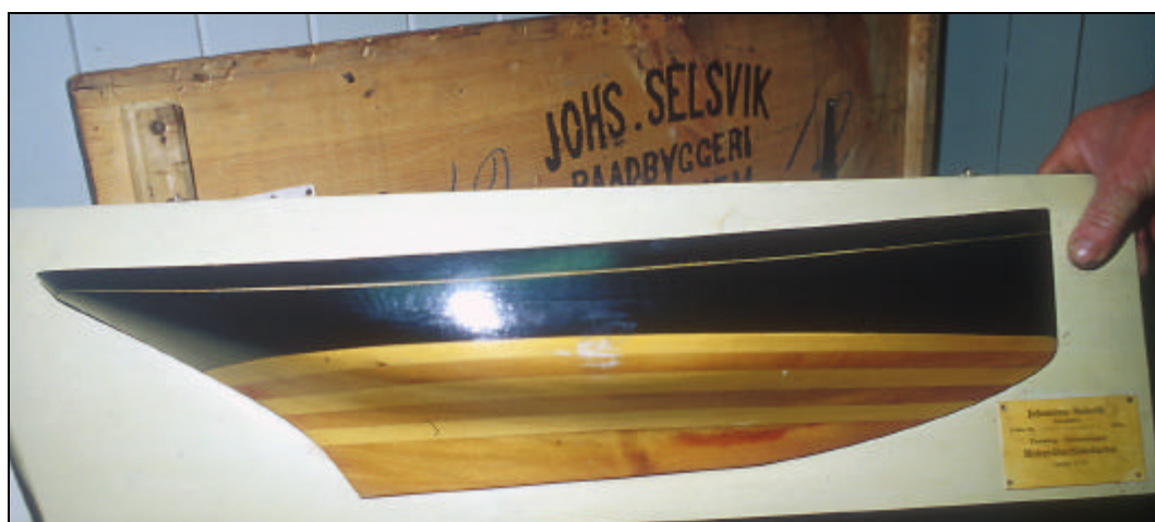
Proposal for a motorized and galley rigged fishing vessel, 70 feet, designed by Selsvik in 1893.
